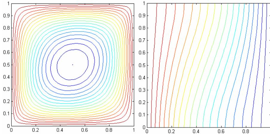
Fig. 3. Streamlines and isotherms for  $Ra = 10$  and  $Q = 0$  (steady state).
