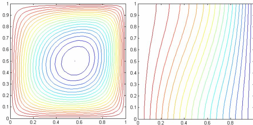
Fig. 4. Streamlines and isotherms for  $Ra = 10$  and  $Q = 1$  (steady state).
