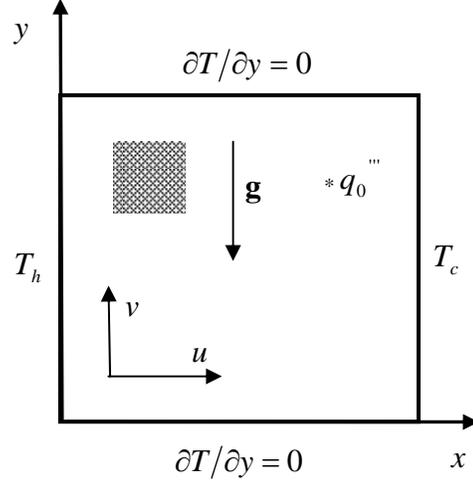
Figure 1. Geometry of the problem and the co-ordinate system, and the boundary conditions.
